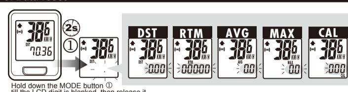
**(\*) :** Current Speed 0-199.9km/h 0-120.0m/h +/- 1%
